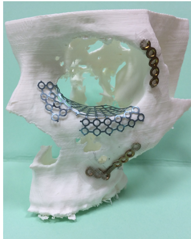
Fig. 2. The resulted 3D model printed with the Flashforge ® Pro Creator, fracture lines and bone defects are drawn on the model. The titanium plates and mesh are shaped according to the patient's specific anatomy.
